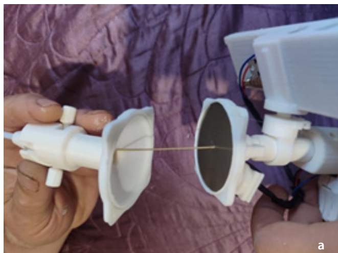
Fig.15. The moment of connecting the replaceable part of the device (A) to the non-sterile base element and memory card view (B)
