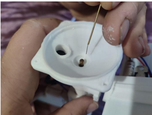
Figure 20. Probe fixed by the collet before closing the noise emission fixation chamber.
