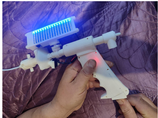
Figure 22. The red indicator on the handle light up, and the base frequency scale appear in the form of a blue bar on the display.
