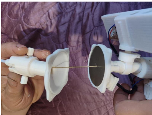
Figure 16. Connecting the sterile replacement part of the device to the base element.
